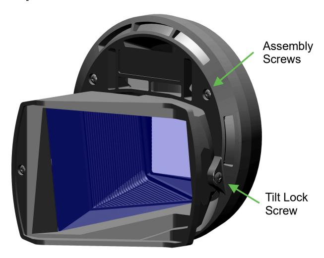
ADJUSTMENTS. Tilt the STE lens in its mount to make any residual image top curvature the same but opposite that at the bottom. Make final adjustments to projector zoom and vertical lens shift to produce the best fit of the image to the screen. Lock the STE lens tilt by tightening the single Phillips tilt lock screw (do not over tighten). As desired you may want to adjust the panel alignment in the projector (see Sony instruction manual).
