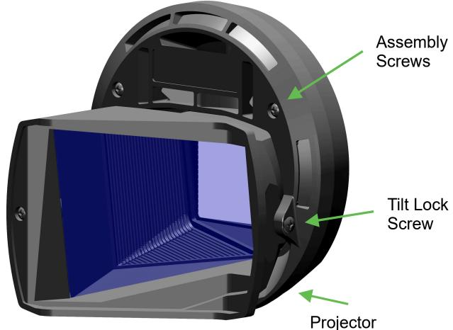
**ADJUSTMENTS.** Tilt the STE lens in its mount to make any residual image top curvature the same but opposite that at the bottom. Make final adjustments to projector zoom and vertical lens shift to produce the best fit of the image to the screen. Lock the STE lens tilt by tightening the single Phillips tilt lock screw (do not over tighten). As desired you may want to adjust the panel alignment in the projector (see Sony instruction manual).
