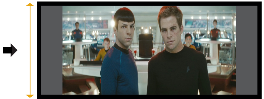
2.40:1 movie is vertically stretched by the projector or scaler to fill the 16:9 area.
