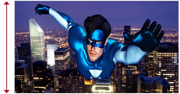
2.40:1 movie is vertically stretched by the projector or scaler to fill the 16:9 frame and use all 1920x1080 pixels
